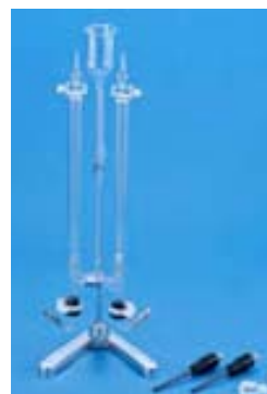
Fig.1 Hoffman Electrolysis Apparatus
