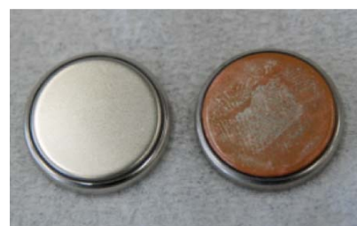
Fig. 7 Cathode surfaces (before/after reaction )
