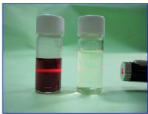
Figure 2. The colloidal AuNPs solution (left) presented the Tyndall effect, while the HAuCl 4 solution with the behavior of a true solution (right) does not.
