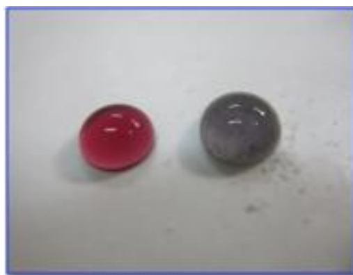
Figure 3. The aggregation of AuNPs by adding granular sodium chloride to change color from ruby red to dark gray, at the right side of a liquid ball.
