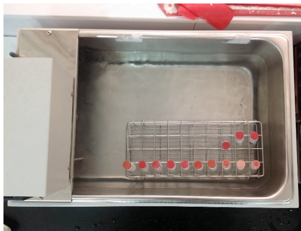
Figure 4. New prepared storm glasses were placed in a thermostatic water-bath
