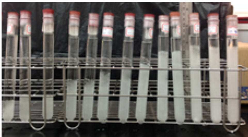
Figure 11. The height of precipitation with different ratio of ethanol in the storm glass at 16 °C.
