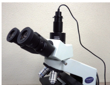
Figure 5. The imager being mounted to the microscope Left side: microscope CX21 Right side: microscope YM-400LR
