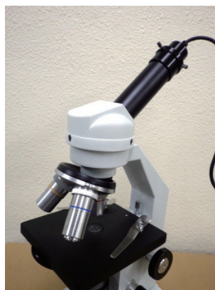
Figure 5. The imager being mounted to the microscope Left side: microscope CX21 Right side: microscope YM-400LR
