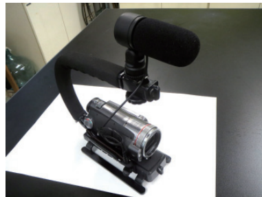
Figure 2. The digital High-Vision camera HDC-TM350 and the microphone ME-1 attached to the stabilizer X-Grip unit.
